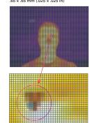
If you set up a 640 × 480 resolution infrared camera about 1 meter from a subject, the resulting image plane would be 418 x 312 mm (16.45 × 12.28 in). Therefore, a single pixel would have a spot size of .65 × .65 mm (.025 × .025 in).
