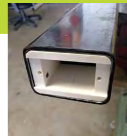
Extensive laboratory work verified the validity of the ICPT concept, and beta field test ensued. Technical staff at San Diego integrator Door Systems, Inc., worked out frame mounting details for removable mullions with the creative use of a 3-D printer.
