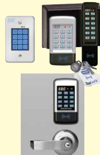
keypads designed to control access of a single entry point for facilities with up to 500 users. Each user is assigned a personal identification number (PIN). Keypad entry of a valid one to six digit code activates one or both of the output relays which releases an electric door lock. Optional Prox Readers are available for selected 920 and 923 models.
