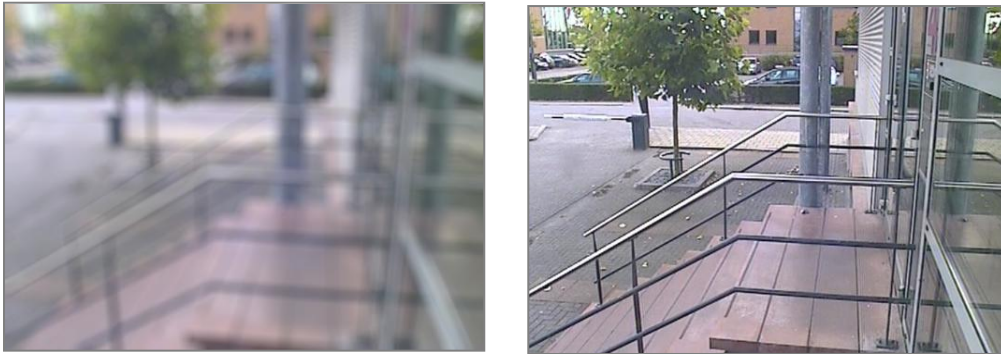
Figure 3 Unfocused image (left); focused image (right). The focus measurement alerts operators the moment pictures start to look blurry.
