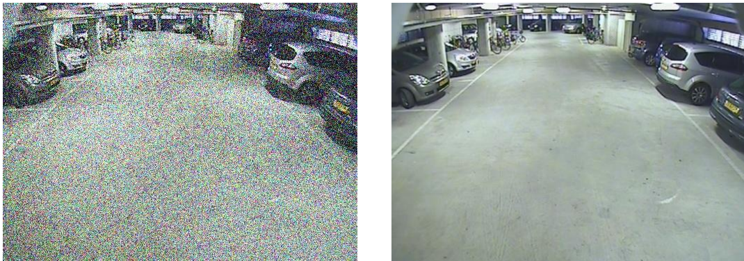
Figure 7 Too much noise (left); a balanced signal to noise ratio (right)
