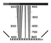
Resolution test charts have "wedged" line patterns. The resolution is measured at the last point where the lines are visually discernable.
