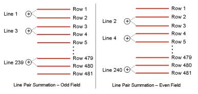
CCD sensors capture interlaced video using a process called line pair summation that eliminates flicker but throws away 25% of the vertical resolution.
