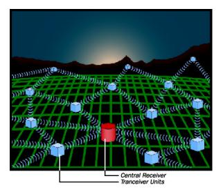
The Central Receiver is the primary receiving location of the data for the network. The Central Receiver is a computer platform that integrates network management software and related applications to maximize network management. Each box indicates an SST in a remote location that sends and receives data from the Central Receiver and other SSTs to insure a dynamic data path, which optimizes information flowing reliably across the network on a continual basis.
